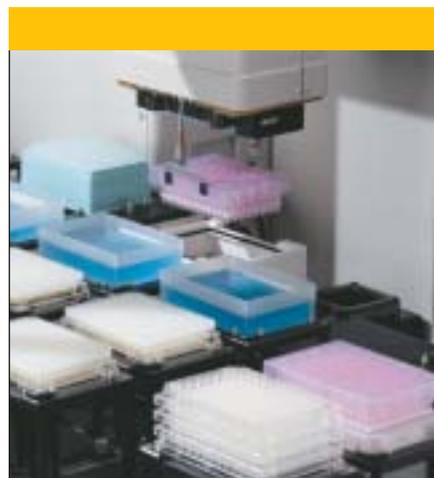
**Figure 4:** A gripper arm configured on a liquid handling workstation (Biomek FX) moves microplates into and around its deck and assembles and disassembles a vacuum block used for liquid processing through plates. (Courtesy of Beckman Coulter.)
